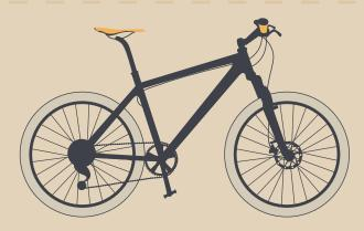
**MOUNTAIN BIKE:** Made for off-road cycling with features like large, knobby tires, durable wheels, front or full suspension, powerful brakes, and a variety of gear ratios to enable climbing and descending steep slopes.
