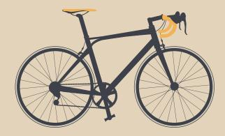
**ROAD BIKE**: Built to handle paved roads. Tires are narrow with highpressure and smooth surfaces to decrease resistance. Handlebars are dropped. Many have derailleur gears, but there are single speed and fixed gear models available.
