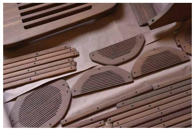
From design to completion, each Streblow is customized to the owner's specifications. All parts and components, including these speaker grills and decorative accents made of teakwood are fabricated to the boat's plans. Only one new Streblow a year is built.
